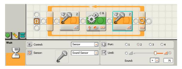
5. Add a second "Move" block, setting it to stop motors A and B.
