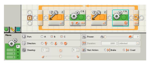
6. Add a third "Wait" block, programming it to wait for the sound sensor to read a value of less than 48. (This allows for the sound of a loud clap to die down so that it does not retrigger the first "Wait" block, causing the motor to stop very briefly but then move again when the loud clap is made.)
