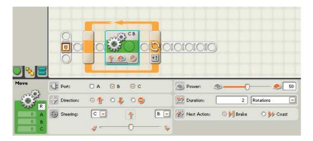
3. Add a second "Move" block after the first one in the loop, setting it to move motors B and C (or whatever ports your motors are attached to) to the right for 90 degrees.
