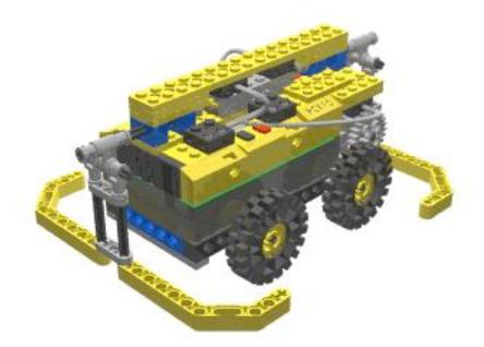
*Hint: Since the surface area of the touch sensor is small, build bumpers to increase its sensitivity (larger surface area).*
