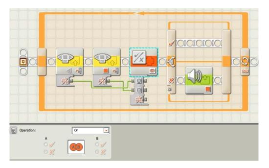
3. Insert a third "NXT Buttons" block after the logic block you just added. Set this "NXT Buttons" block to the Right button, when pressed. Add another "Logic" block after this "NXT Buttons" block, set to Or. Wire in the true/false output from the Right button "NXT Buttons" block to input A on the "Logic" block. Wire the result from the first "Logic" block to input B of the second "Logic" block. Then, wire the result from the second "Logic" block to the switch's input.
