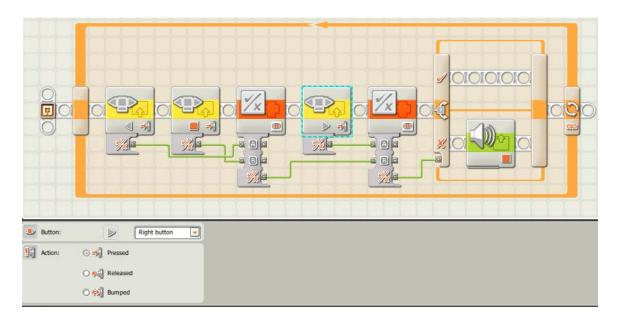
4. On the switch's true, or upper, beam, add a "Touch Sensor" block set to port 1, when pushed. Add a second "Touch Sensor" block set to port 4, when pushed. Add a "Logic" block set to Xor. Wire the true/false outputs of both "Touch Sensor" blocks to inputs A and B of the Xor "Logic" block.
