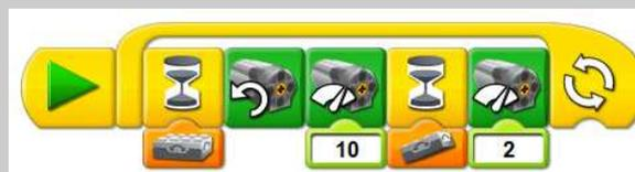
This program uses the motion sensor to determine the speed of the car. If the tilt sensor is tilted upwards, the car will slow down and if the tilt sensor is flat, the car will travel faster.
