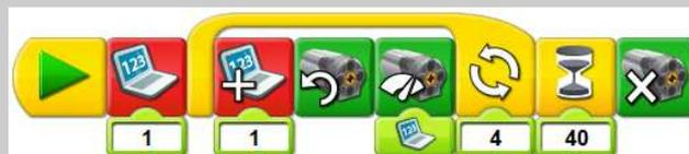
This program can be used to accelerate the car up the ramp. Starting from rest creates enough traction to stop the car from slipping.
