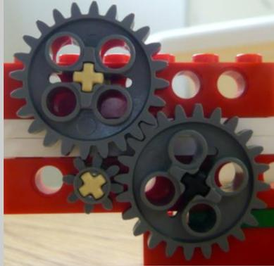
5. Give each student pair the task of building a gear system that incorporates one of the following: crown gears, worm gears, gearing up, gearing down, idler gears, or tooth rack gears. Allow 10 minutes for building.
