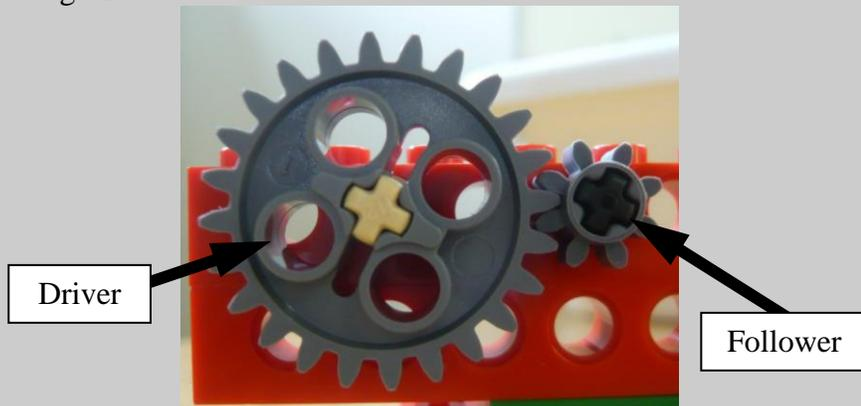
3. Ask them if they have an idea of what an idler gear does. Explain that the idler gear is used to change the direction of the next gear and does not change the speed of the follower gear in relation to the driver gear.
